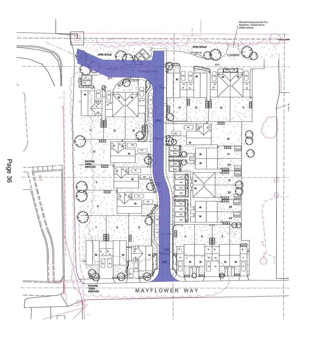
EASEMENT TO SHOW POINTS OF CONNECTION FOR CLT ONTO THE ESTATE ROAD FOR FOUL SEWER
